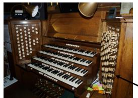
The console has 4 keyboards, these are called **manuals**. When the organist presses the keys on the manuals, air is sent through different pipes. A **blower** pumps air into the organ. Today this is electric, but a long time ago hand operated bellows were used.
