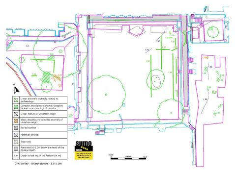
Figure 5: Interpretation of the GPR data from 1.5m-2.3m.
